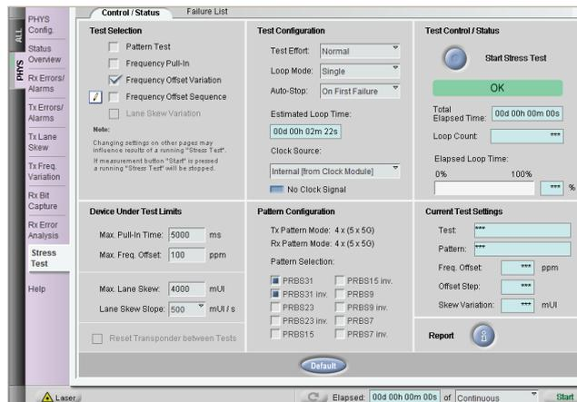
Figure 6. CFP2 stress test
