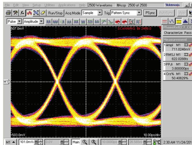
Figure 8. Timing margins at 25 G are extremely tight and require low jitter triggers and low phase-noise clocking.
