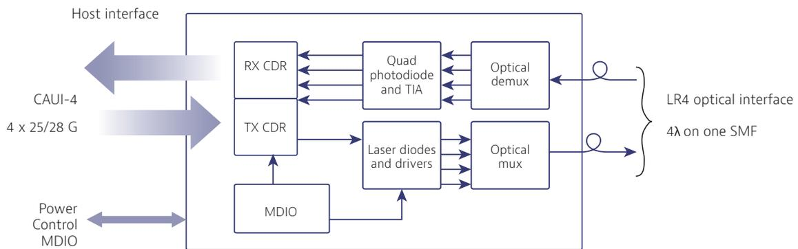
Figure 2. CFP2 Block Diagram
