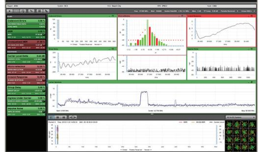
Increased utilization of upstreams makes it abundantly clear that spectrum-analysis-only-based tools can no longer manage the task of service/network maintenance alone. The biggest changes in the (Data over Cable Interface Specification) DOCSIS® 3.0 environment are upstreams crowded with wider carriers and higher-modulation quadrature amplitude modulation (QAM) carriers with increased sensitivity to impairments.
