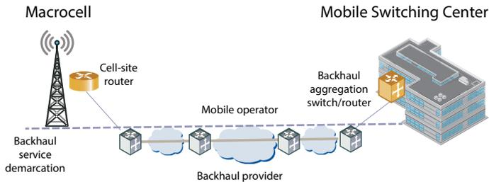
Figure 1. Macrocell mobile-backhaul reference network
