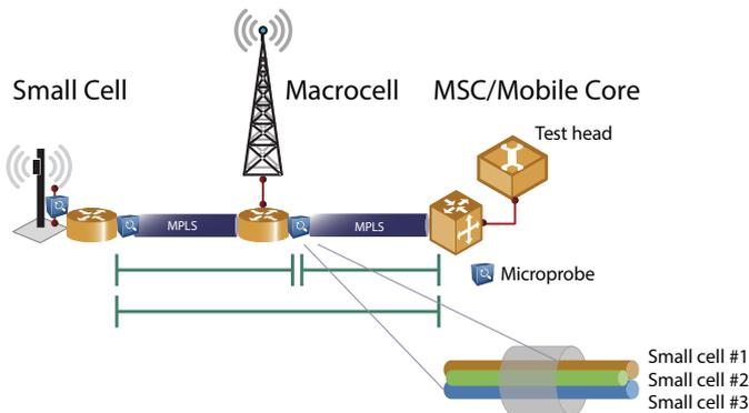
Figure 9. Microprobes deployed along the full service delivery path
