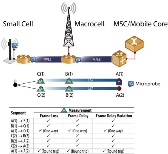
Figure 10. Microprobes provide segment-by-segment one-way latency measurements
