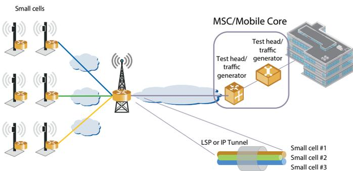
Figure 3. Small-cell backhaul hub-and-spoke topology
